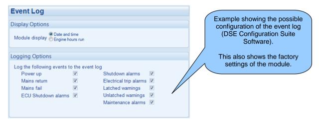
Once the log is full, any subsequent event overwrites the oldest entry in the log. Hence, the log always contains the most recent events. The module logs the alarm, along with the engine running hours.
