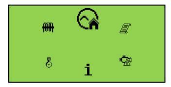
To select the required icon, press the (up) button to cycle right or the (down) button to cycle left until the desired instrumentation section is reached.
